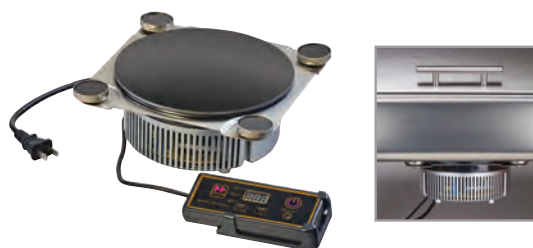
D. MAGNETIC INDUCTION CHAFER ATTACHMENT Converts Chafers with Easy Access Drawers into Flameless Induction Units. Stainless Steel Piece is Placed in Water Pan, Unit Attaches Magnetically Below. ITEM 4011 | 8¼Wx8¼Dx3½H
